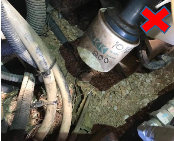
Rock and dirt build up in engine bay
