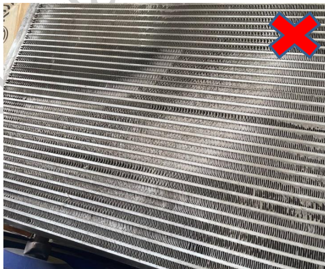
Bent Fins and Debris Damage
