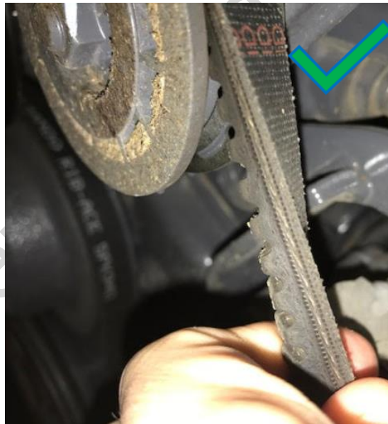
Belt is correct tension and water pump spins freely
