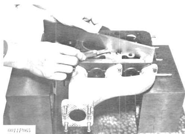
Fig. B-33 Checking Distortion of Cylinder Head Surface
