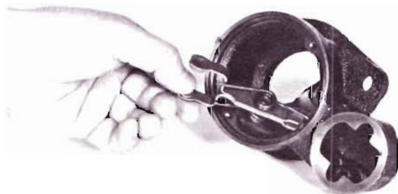
Fig. N-41 Detaching Drive Lever
