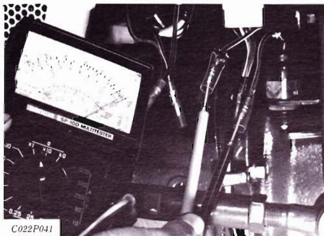
Fig. N-43 Checking Safety Switch
