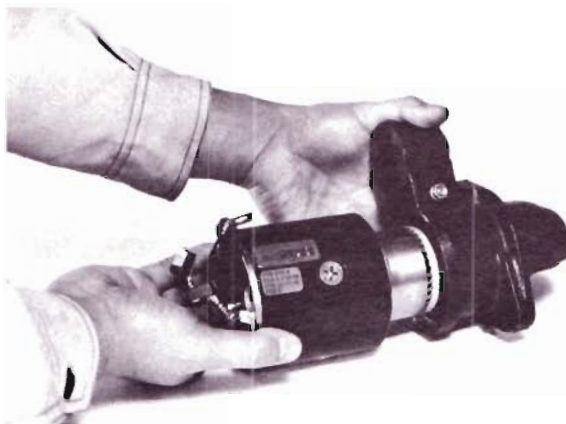
Fig. N-39 Removing Yoke
