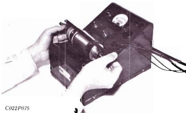
Fig. N-55 Checking Armature Coil Short-circuit
