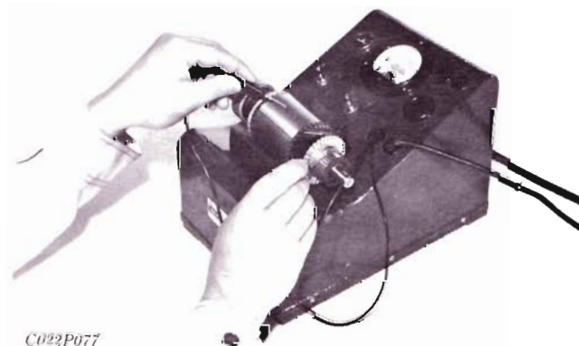
Fig. N-57 Checking Armature Coil Grounding
