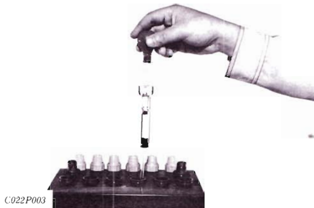
Fig. N-20 Checking with a Hydrometer
